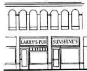
These signs complement the building form and create a more orderly appearance
