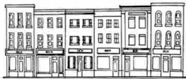
Wall signs of consistent size and placement establish facade rhythm.
